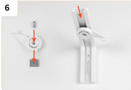
Prepare the wall fixture as shown in Fig. 6, by screwing all components together (depicted on the left). Insert the holder into the angled mounting (depicted on the right). Please note: When you fasten the holder, you should still be able to turn it.
