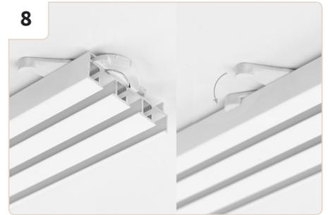
Begin with the installation of the leftmost track rail. The lever is oriented towards the wall. Lift the track to the ceiling so that the fixture sits in the groove on the upper side of the rail. Turn the lever counterclockwise until the track rail is secured.
