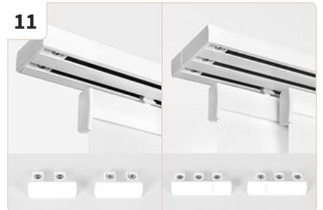
Insert the panel curtains into the tracks in the desired order. Separate the required end cups and fasten them with a screw on the two ends of the rails.
