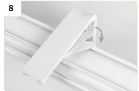
Begin with the installation of the leftmost track rail. The lever is oriented towards the wall. Lift the track to the ceiling so that the fixture sits in the groove on the upper side of the rail. Turn the lever until the track rail is secured.
